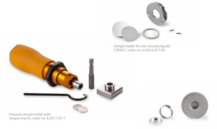
Sample container made of Al, specifically for easy preparation of waxes, order no. 6.256.4-91.6.00
