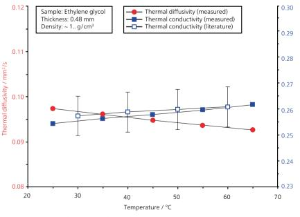
Thermal diffusivity and thermal conductivity of an engine coolant
