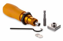
Torque wrench for pressure sample holder, included in order no. 6.257.1-91.9.00
