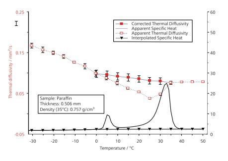
LFA and DSC measurement into the melting range of paraffin
