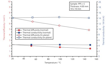
LFA 427 measurement on a PPS+C sample in the sample holder for lamellar samples
