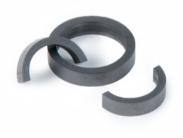
Sample holder for fibrous samples made of graphite, order no. 6.256.1-93.6.00, but also available in  $Al_2O_3$ , order no. 6.256.1-93.3.00.
