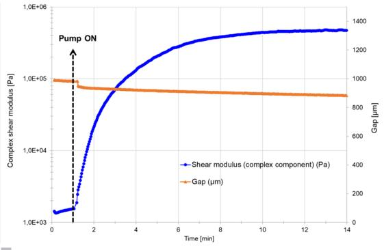
2 Complex stiffness and gap during paint drying
