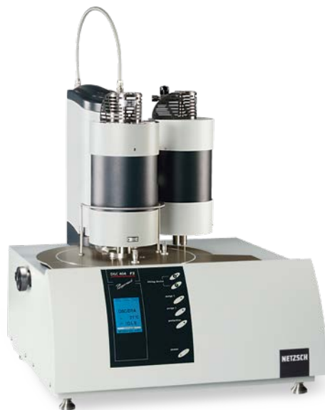
DSC 404 F1/F3 Pegasus® with two furnaces
