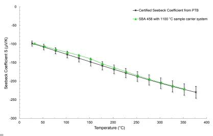
4 Measurement of the Seebeck coefficient of the certified lead telluride, PbTe, with the SBA 458 in comparison with literature - Sources [1] und [2]
