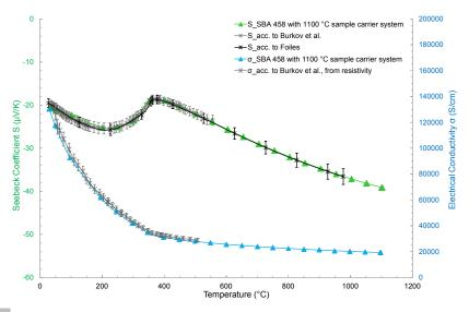
2 Measurement of the Seebeck coefficient and the electrical conductivity of nickel with the SBA 458 in comparison with literature – Sources [1] and [2]
