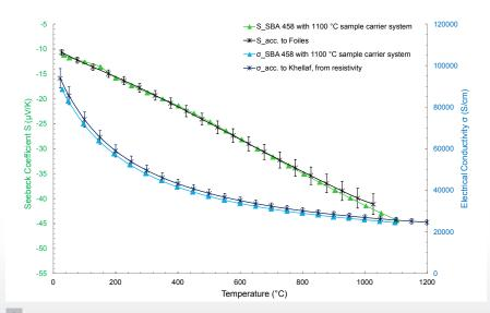
**3** Measurement of the Seebeck coefficient and the electrical conductivity of palladium with the SBA 458 in comparison with literature – Sources [2] und [3]
