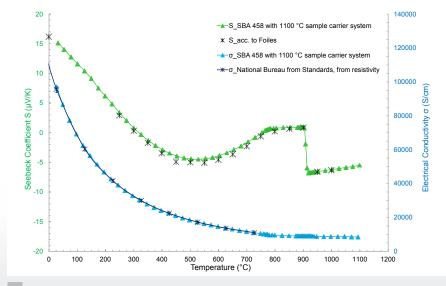
5 Measurement of the Seebeck coefficient and the electrical conductivity of pure iron with the SBA 458 in comparison with literature - Sources [2] and [4]
