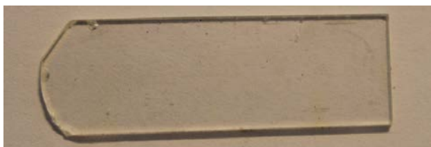
3 Undamaged wafer sample following multiple tests
