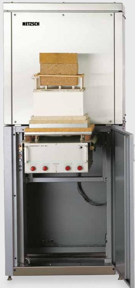
NETZSCH Thermal Conductivity Tester 426
