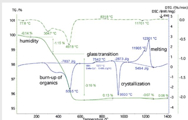
STA measurement of a glass wool sample
