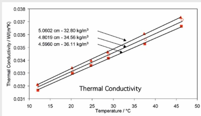
Thermal conductivity of the glass fiber insulation at different loads
