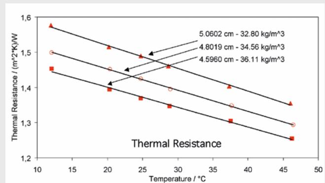
Thermal resistance of the glass fiber insulation at different loads
