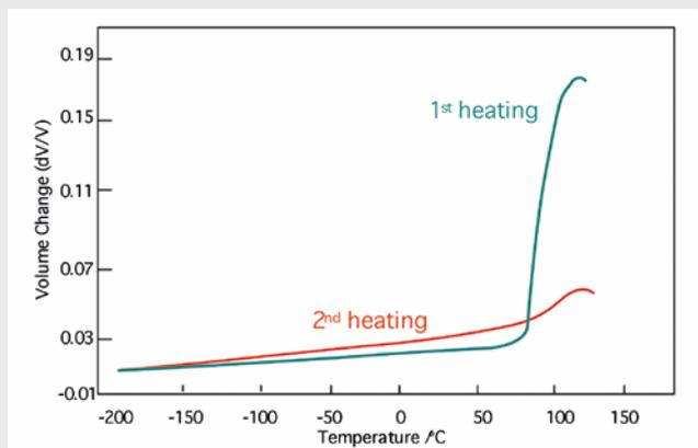
Volume change of polystyrene between -180°C and 140°C measured with the DIL 402 C
