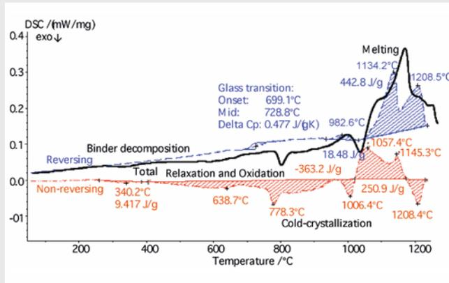
Temperature-modulated DSC measurement of a mineral fiber insulation
