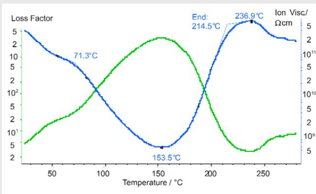
Curing process of mineral wool infiltrated with an uncured resin
