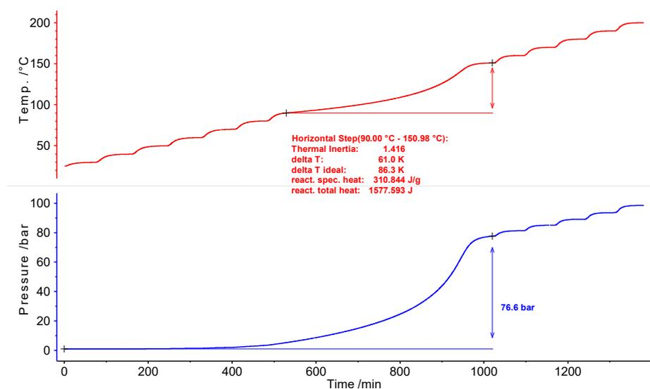
3 HWS results for hydrogen peroxide (17.5%), temperature (red) and pressure (blue)
