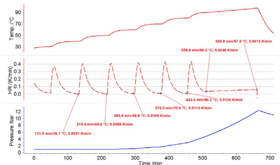
5 HWS results for hydrogen peroxide (17.5%), temperature (top), self-heating rate (middle) and pressure (bottom)
