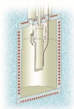
2 Cross-section of the ARC module of the NETZSCH MMC 274 *Nexus*®
