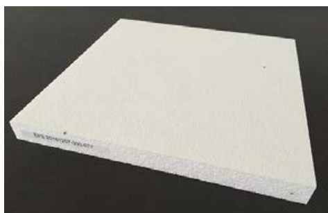
1 Photo of a 300 mm x 300 mm x 25 mm NETZSCH EPS specimen
