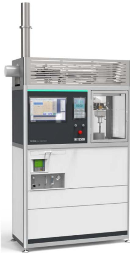
1 Cone Calorimeter TCC 918
