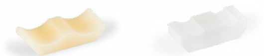
Sample-supporting kits made of alumina and fused silica for double measuring system
