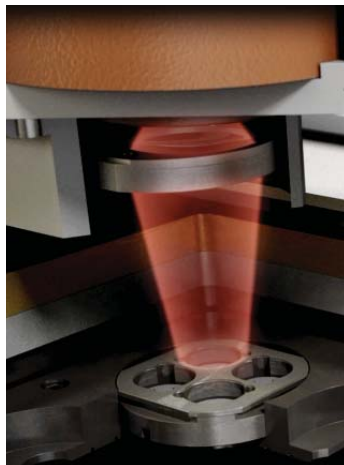
6 Illustration of ZoomOptics and its influence on the measurement results on Pyroceram at RT
