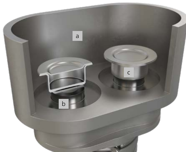
7 Ideal combination of Arena furnace (a), ring-shaped sensor (b) and Concavus crucibles (c). The concave area is an exaggerated image for better illustration purposes; in reality, concavity is only approx. 10 µm.
