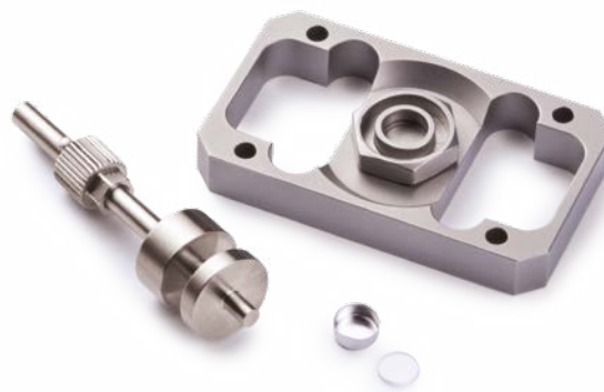
Frame with sample insert, pushrod and sapphire disc for compression measurements on pasty samples. The use of aluminum pans (NGB810405) prevents sample holder contamination.
