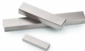
Steel bars for system stiffness calibration
