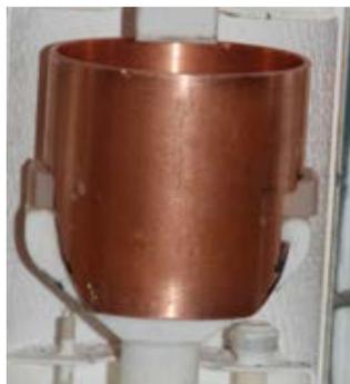
2 Temperature shield of copper (to 950°C), zirconium inset for higher temperatures
