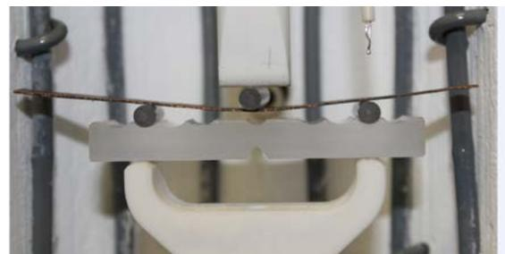
3 Roller bending support with additional gimbal push rod
