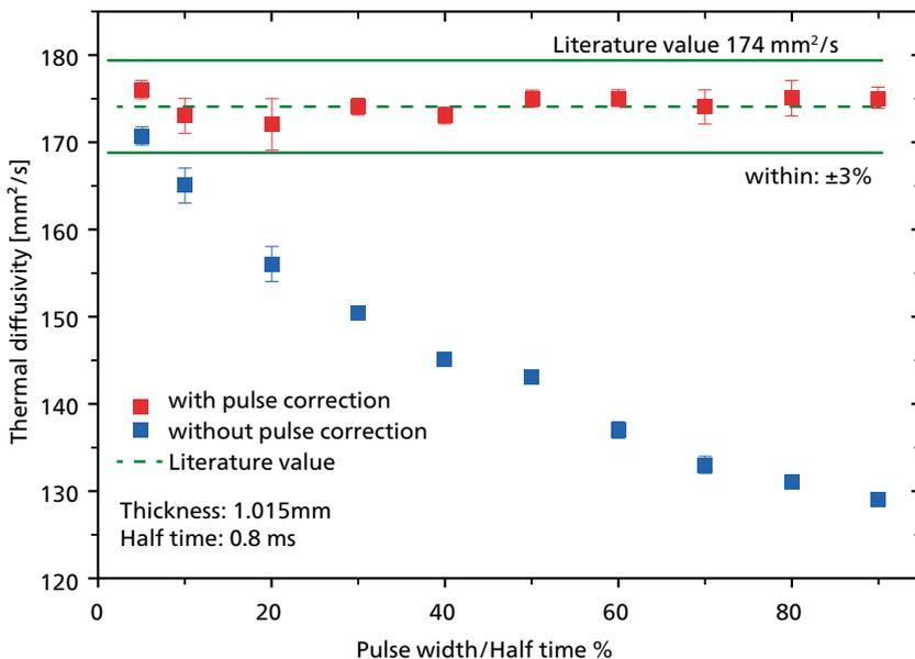
The influence of pulse correction is demonstrated with measurements on a 1.015-mm-thick silver plate at 25°C. This example proves that accurate measurement results are obtained within  $\pm 3\%$  of the literature value when an intelligent pulse correction method is used.
