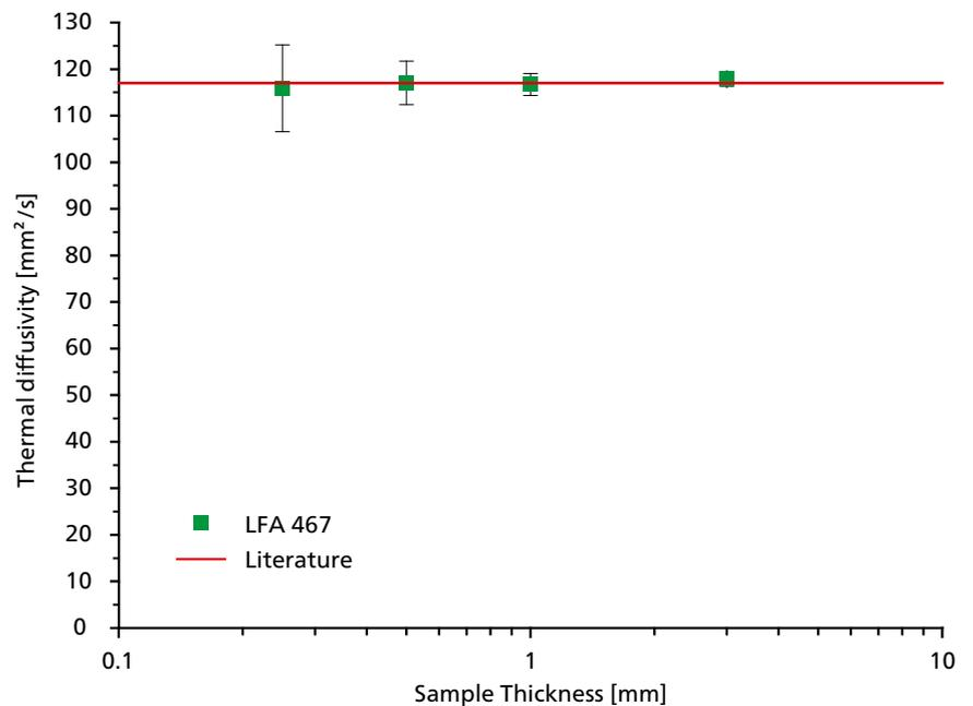
LFA 467 *HyperFlash*<sup>®</sup>: Thermal diffusivity values for the copper samples are in very good accordance with literature data, irrespective of the sample thickness.
