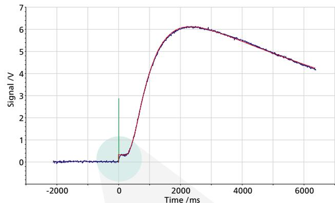
Radiation model:  $0.877 \text{ mm}^2/\text{s}$
