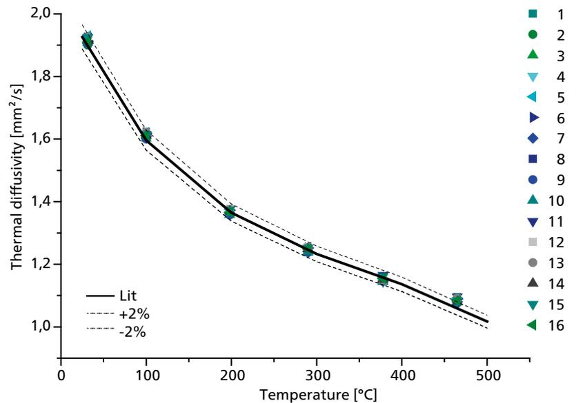
LFA 467 *HyperFlash*<sup>®</sup>: Measurement results of 16 Pyroceram samples (2.5 mm thick, 12.7 mm in Ø) between room temperature and 500°C obtained by one run. The evaluation of the thermal diffusivity shows a deviation of  $\pm 2\%$  from literature data.
