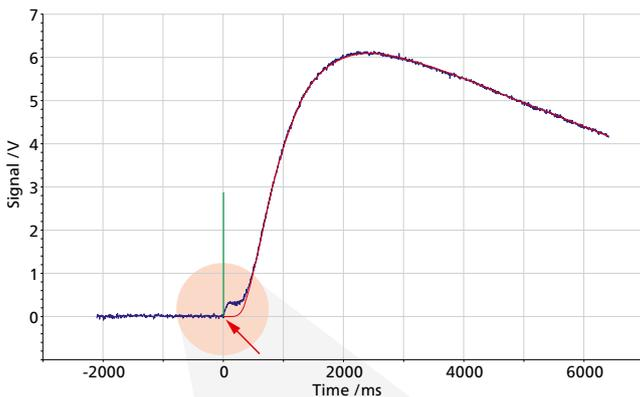
Conventional heat loss model (standard):  $0.974 \text{ mm}^2/\text{s}$
