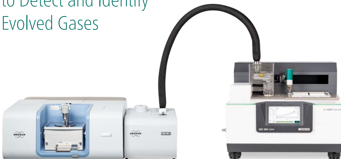
DSC 300 Caliris ® with ASC, coupled to the Bruker FT-IR spectrometer
