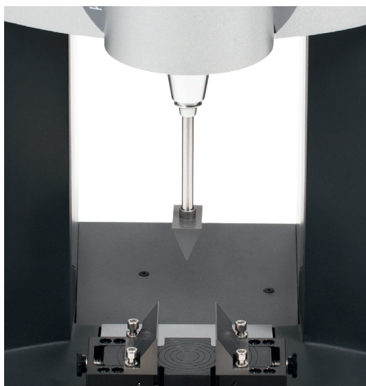
1 Kinexus rotational rheometer equipped with the texture analysis setup for characterizing brittle solids (biscuits, chocolate).
