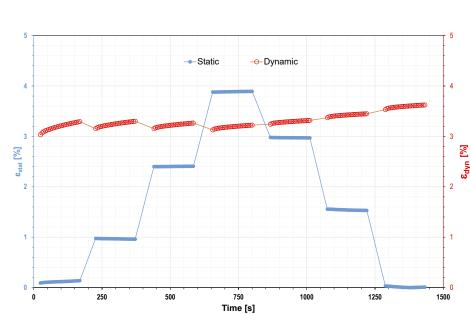
4 Variation of the static and dynamic strain over time for the rubber-metal buffer with one stud bolt and one threaded hole
