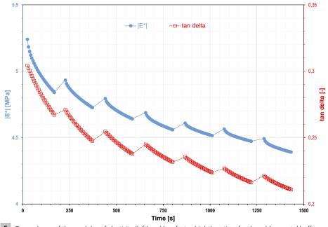
5 Dependence of the modulus of elasticity (left) and loss factor (right) on time for the rubber-metal buffer with one stud bolt and one threaded hole at room temperature and a frequency of 10 Hz
