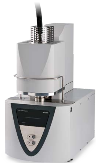
STA 2500 Regulus with transfer line for STA-FT-IR coupling
