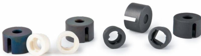
Centering cones and caps for round and square samples (diam. of 10 mm); centering cones made of Al<sub>2</sub>O<sub>3</sub> (white) and graphite (grey); caps made of SSiC and graphite.
