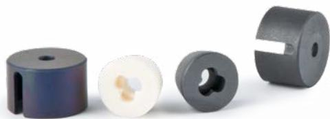
Centering cones and caps for sample of 6 mm diameter; centering cones made of Al<sub>2</sub>O<sub>3</sub> (white) and graphite (grey); caps made of SSiC (left) and graphite (right).
