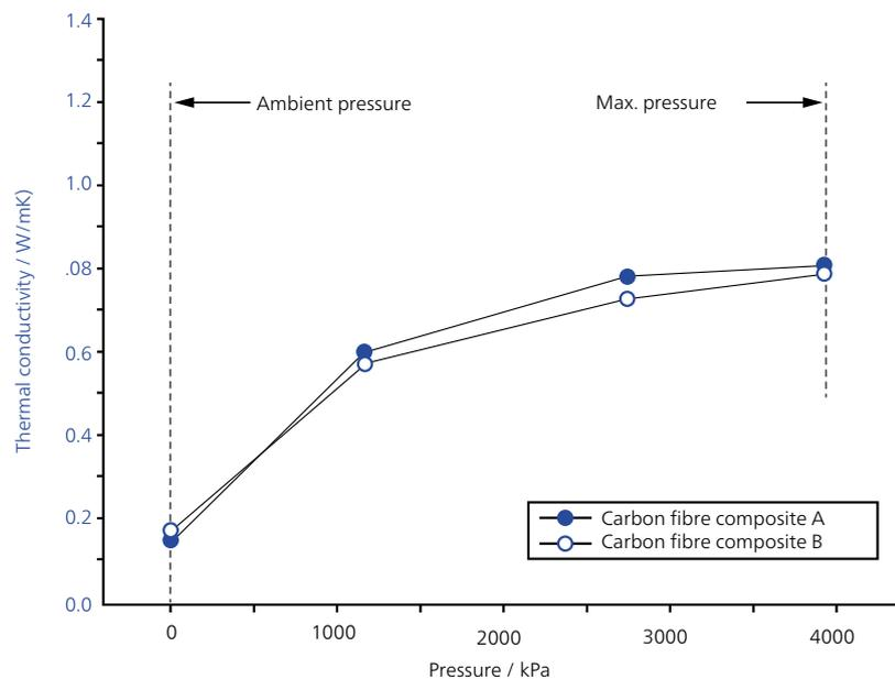
LFA 457 *Microflash*® measurements on two carbon fibers (2 mm thick) between ambient and 4 MPa in air at room temperature.
