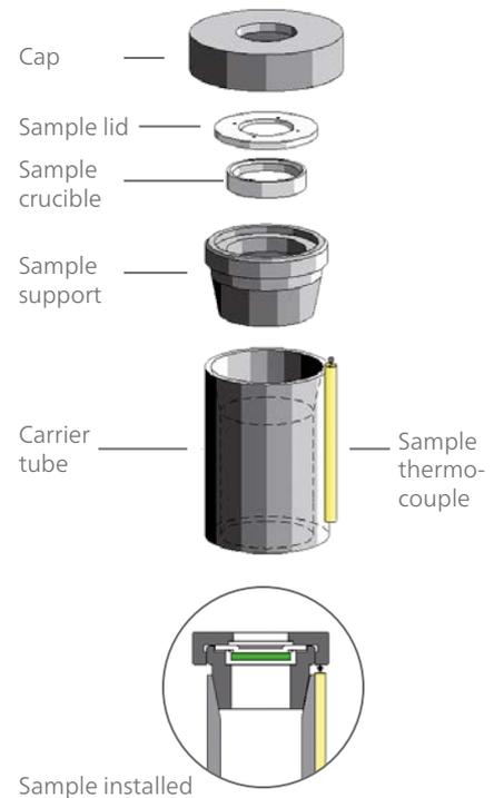
The set up of the sample holder for "liquid metals"\* requires no multi-layer analysis of the test results.
