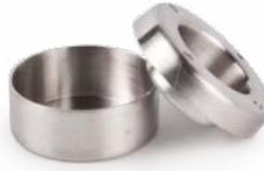
This container fits into sample holders with a diameter of 12.7 mm. Measurements on materials such as phase change materials (PCM) can be carried out in the solid and liquid state, as well as in the range where the phase change occurs.
