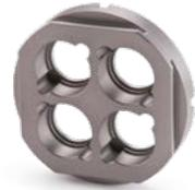
Standard sample holder, 12.7 mm diameter, order no. LFA46700A90.011-00
