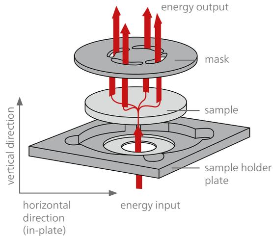
Heat flow directions using the in-plane sample holder. The special set-up of the in-plane sample holder eliminates the typical measurement limitations caused by the minimum sample thickness.
